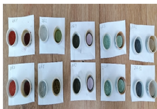
Fig. 1 Initial mixtures and synthesized pigments: in each composition the mixture is on the left, and the pigment synthesized at 1200°C is on the right
