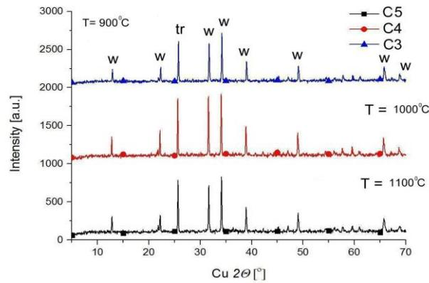
Figure 7. XRD parents of Co - doped (0,375CoO) zinc silicate annealed at 900, 1000 and 1100 °C. Legend: w- willemite, tr- trydimite (SiO<sub>2</sub>)
