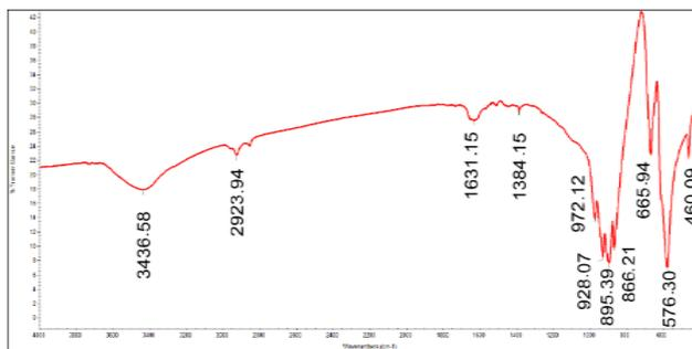
Figure 10. FTIR spectrum of composition C2 (CoO.ZnO.SiO<sub>2</sub>)
