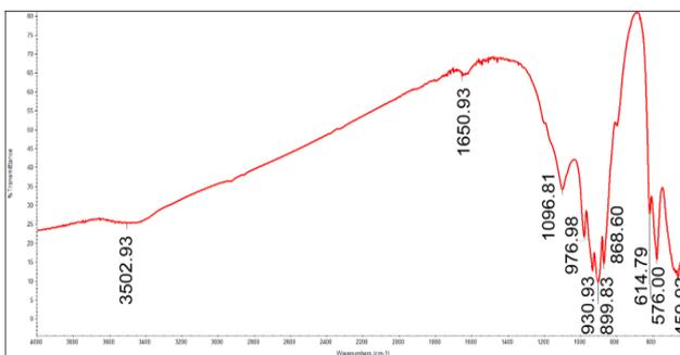
Figure 11. FTIR spectrum of composition N2 (NiO.ZnO.SiO<sub>2</sub>)
