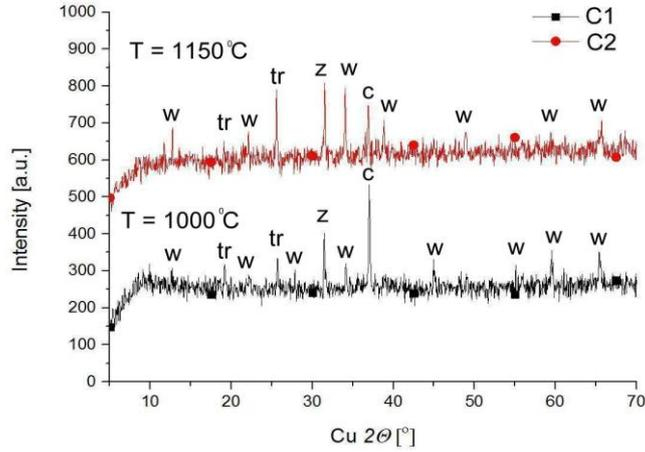
Figure 6. XRD parents of Co - doped zinc silicate annealed at 1000 and 1150 °C. Legend: w- willemite, tr- trydimite (SiO<sub>2</sub>), z- ZnO, c- CoO
