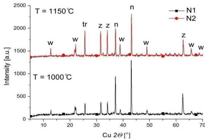
Figure 8. XRD parents of Ni - doped zinc silicate annealed at 1000 and 1150 °C. Legend: w- willemite, tr- trydimite (SiO<sub>2</sub>), z- ZnO, n - NiO
