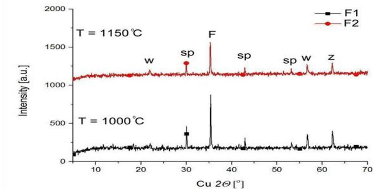
Figure 9. XRD parents of Fe - doped zinc silicate annealed at 1000 °C and 1150 °C. Legend: w- willemite, sp- spinel ( $ZnO \cdot Fe_2O_3$ ), z- ZnO, f-  $Fe_2O_3$
