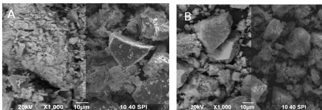
**Figure 4.** SEM of pigments with composition: A) 0,375CoO.1,625ZnO.SiO<sub>2</sub>, B) 0,375NiO.1,625ZnO.SiO<sub>2</sub>
