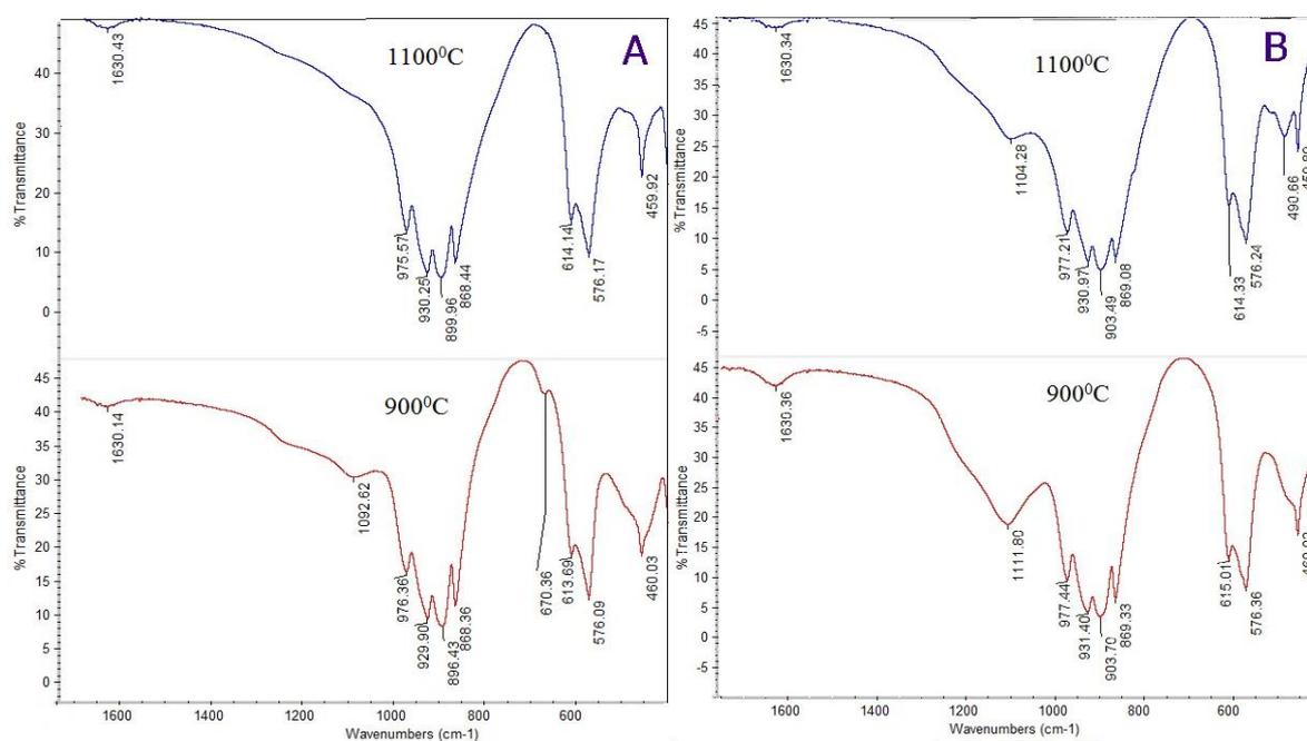
**Figure 2.** FT- IR spectra of pigments  $0,375\text{CoO}.1,625\text{ZnO}. \text{SiO}_2$ (A) and  $0,375\text{NiO}.1,625\text{ZnO}. \text{SiO}_2$  (B)
