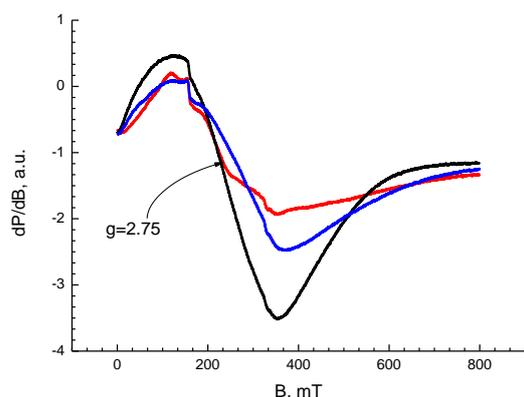
**Figure 3.** ESR spectrum of the sample  $0.5\text{CoO}.1.5\text{ZnO}.\text{SiO}_2$  at 295 K (black curve), 210 K (blue curve) and 120 K (red curve).
