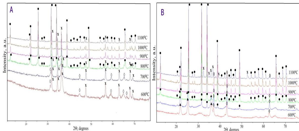
**Figure 1.** A) X – ray spectra of willemite pigments with composition  $0,375\text{CoO}.1,625\text{ZnO}.\text{SiO}_2$  synthesized at temperature:  $600\text{--}1000^\circ\text{C}$ , main phases: ● – Co willemite ; x - zincite  $\text{ZnO}$ ; ◇ -  $\text{Co}_3\text{O}_4$
