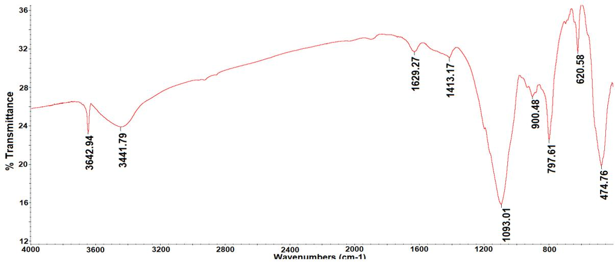
Fig. 7. IR spectrum of blend 3 sintered at 1000°C
