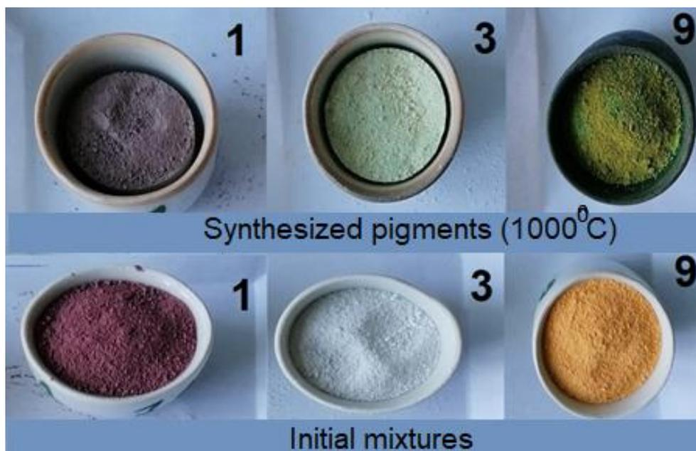
Fig. 1. Initial blends and sintered pigments - synthesized at 1000°C
