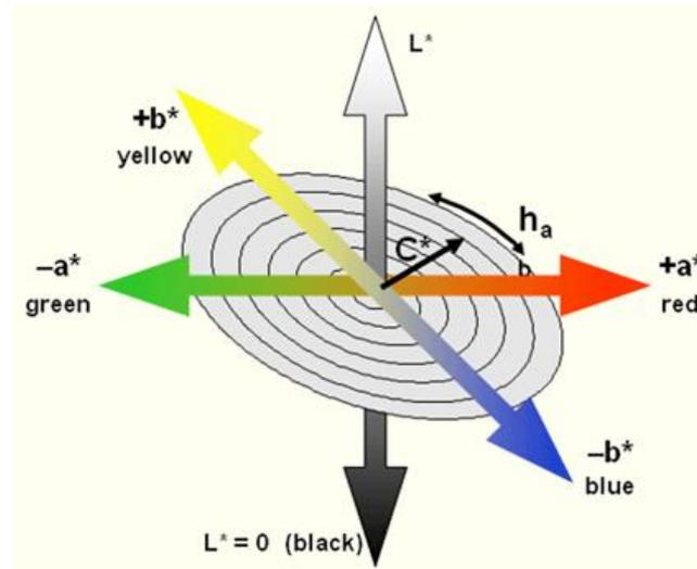
Fig. 2. Colour space of CIELab system
