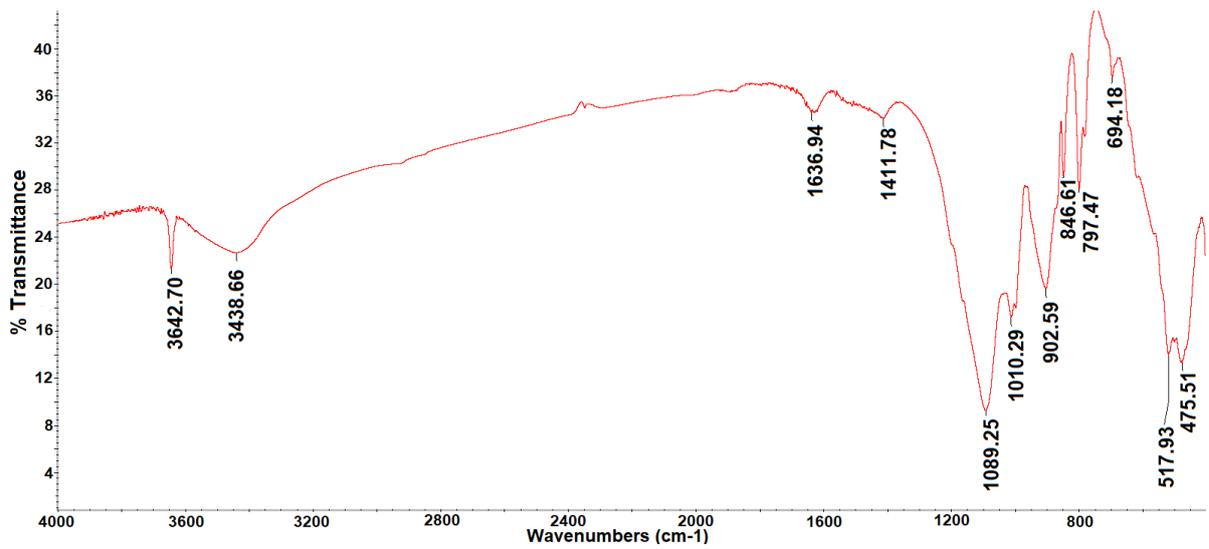
Fig. 6. IR spectrum of blend 1 sintered at 1000°C
