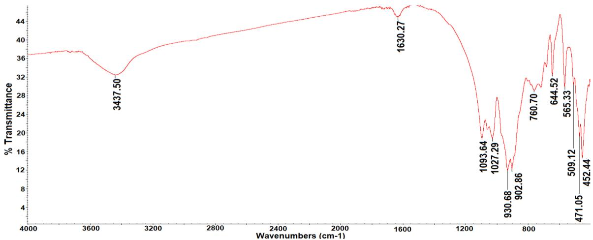
Fig. 8. IR spectrum of blend 9 sintered at 1000°C
