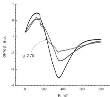
The single anti-symmetric signal determined at 295 K is typically contributed to high-spin exchange bonded  $\text{Co}^{2+}$  in a field with an octahedral distortion [13].
