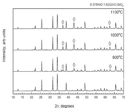
The performed analysis reveals that even at 900 °C are present peaks of the main phases- willemite, solid solution between willemite and residual NiO.
